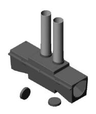
When the vertical tubes are not used, it is also quick and easy to monitor bait take/trap activation by removing one of the two caps in the top of the box.
